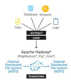
Figure 2. With Apache Hadoop\* software, the ETL (extract, transform, and load) process becomes ELT (extract, load, and transform). The ELT process extracts data from multiple sources and loads it into Hadoop, which then transforms and processes it.
