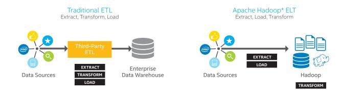
Figure 1. Intel IT evaluated Apache Hadoop\* software as an option for performing traditional ETL (extract, transform, and load) functions. Using Hadoop, ETL becomes ELT (extract, load, and transform), with Hadoop processing and transforming the data at the end of the process.
