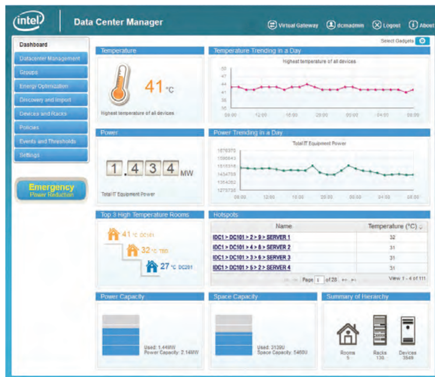
Figure 2. The summary view from the Intel® Data Center Manager (Intel® DCM) management console provides a snapshot of a data center's power and thermal conditions. The Intel DCM provides actual validated data rather than industry estimations or nameplate numbers.
